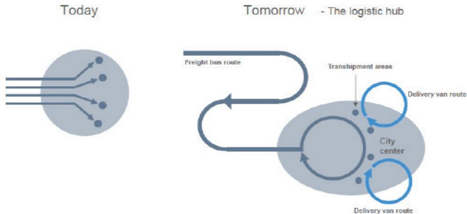
As urban areas grow, there is a need to design better systems for freight and package delivery into urban centers. One proposal is to use a structure similar to bus rapid transit (BRT) systems or even to use the same routes as BRT. This would have large trucks run a circular route, dropping off freight at terminals where smaller trucks would make local deliveries. Figure 12-4 compares the freight delivery pattern of today's system with a proposal for the future modeled after BRT systems.
